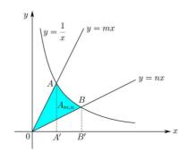
$$\begin{split} A_{m,n} &= S' + \Delta \, OAA' - \Delta \, OBB' \\ &= \int_{-\frac{1}{\sqrt{m}}}^{\frac{1}{\sqrt{n}}} \frac{1}{x} dx + \frac{1}{2} \frac{1}{\sqrt{m}} \sqrt{m} - \frac{1}{2} \frac{1}{\sqrt{n}} \sqrt{n} \\ &= \left[\ln x\right]_{-\frac{1}{\sqrt{m}}}^{\frac{1}{\sqrt{n}}} = \ln \frac{1}{\sqrt{n}} - \ln \frac{1}{\sqrt{m}} = \frac{1}{2} \ln \frac{m}{n} \end{split}$$
