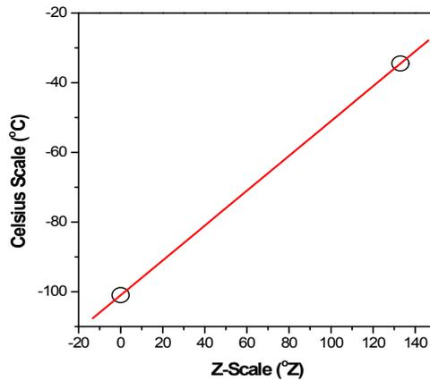
$$\text{기울기} = \frac{-34.5^{\circ}\text{C} - (-101.0^{\circ}\text{C})}{133^{\circ}\text{Z} - 0^{\circ}\text{Z}} = \frac{1^{\circ}\text{C}}{2^{\circ}\text{Z}}$$
